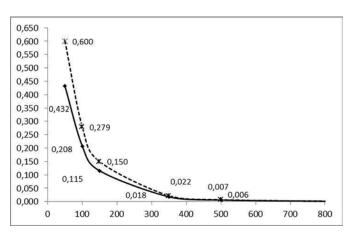
Fig. 3. Probabilities that the rotor line of electric motors manufacturing system is at state 2 and at state 1 or above at time t.
